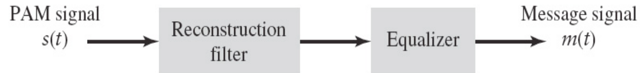
FIGURE 5.7 Recovering the message signal m(t) from the PAM signal s(t) .
