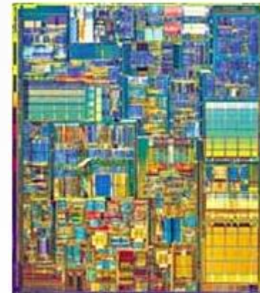
2011 Intel i7 (560,000,000 transistors, 296mm 2 )
