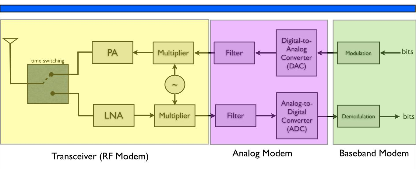
• RF block is characterized by "noise figure" and "gain"
