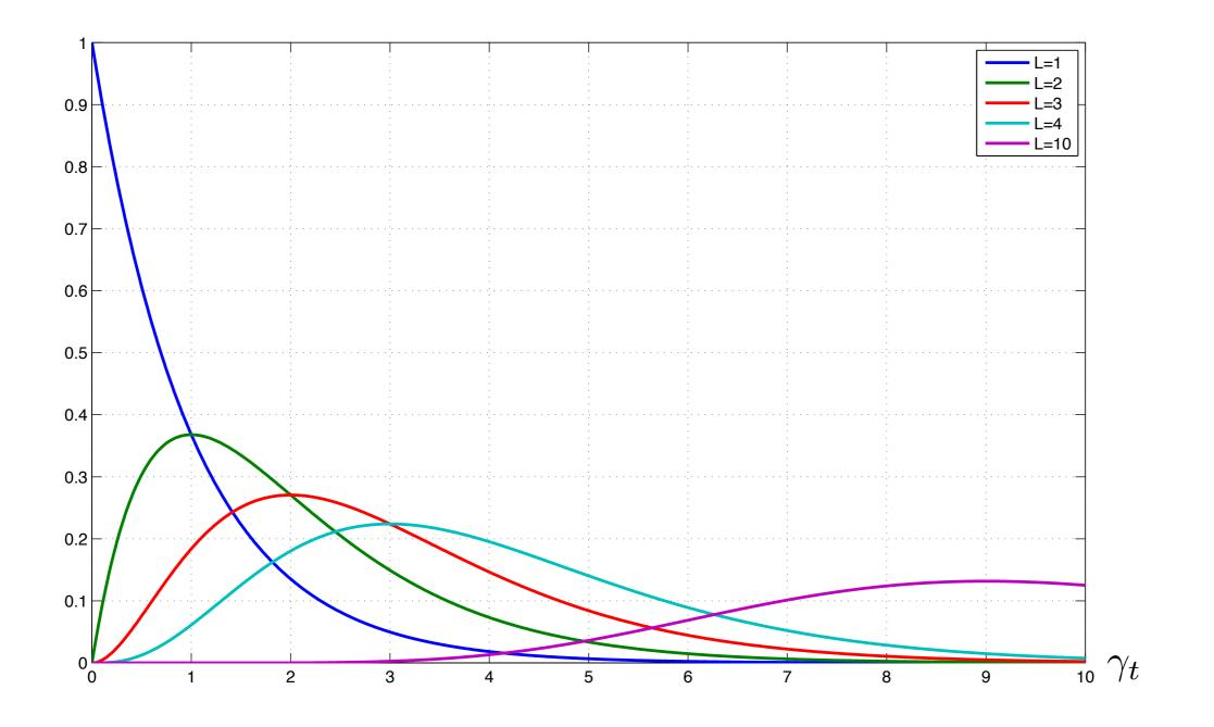
• PDF of the combined output SNR  $\gamma_t$  for L branches CLTD
