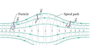
$v_{\parallel} = v \cos \phi$  Straight motion  $v_{\perp} = v \sin \phi$  Circular motion
