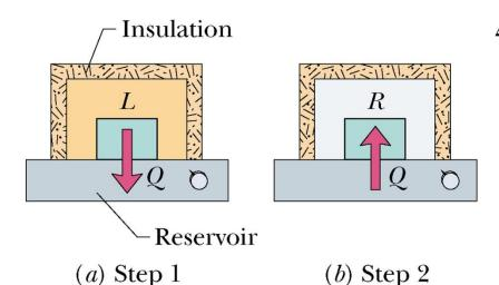
$$\Delta S = \Delta S_L + \Delta S_R = mc \ln \frac{T_f^2}{T_{iL}T_{iR}}$$
