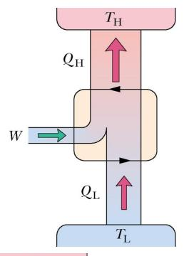
Refrigerator  $COCH. of Performance <math display="block">WS719 작동계수 K = \frac{|Q_L|}{|W|}$
