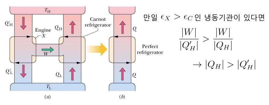
$$W = |Q_H| - |Q_L| = |Q'_H| - |Q'_L| \to |Q_H| - |Q'_H| = |Q_L| - |Q'_L| = Q > 0$$
