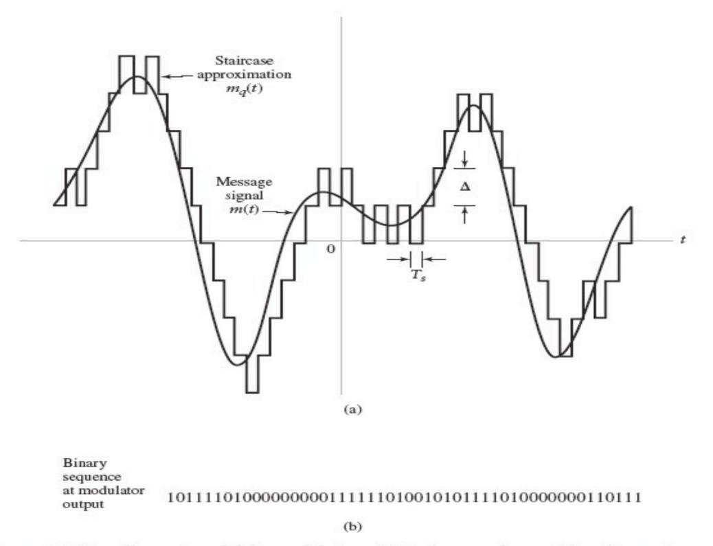
**FIGURE 5.14** Illustration of delta modulation. (a) Analog waveform m(t) and its staircase approximation  $m_q(t)$ . (b) Binary sequence at the modulator output.
