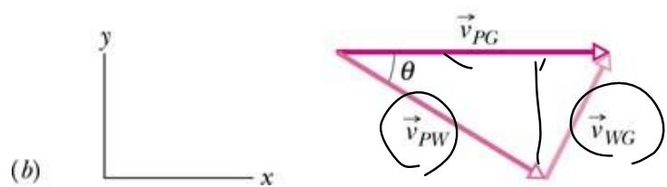
$$\vec{v}_{PG} = \vec{v}_{PW} + \vec{v}_{WG}. \quad (4-46)$$
