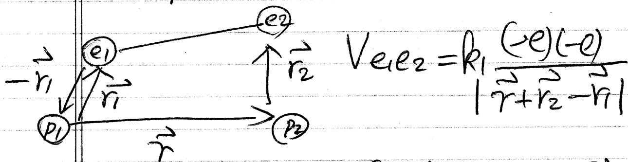
$$V_{e_1 e_2} = k_1 \frac{(-e)(-e)}{|\vec{r} + \vec{r}_2 - \vec{r}_1|}$$
